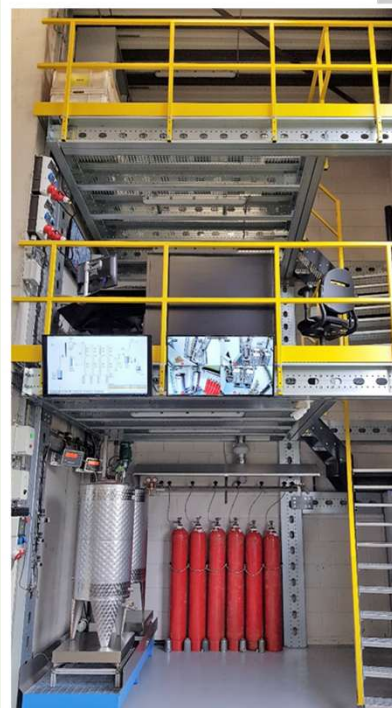
PDU • 20 – 50 kg feed/day • 24/5 operation • Cumulative > ~4,000 h
