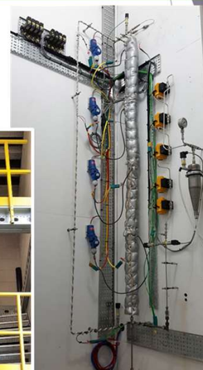
Lab-scale hydrotreaters (5 units): • 0.5 – 1.5 kg feed/day • 24/7 operation • Cumulative > 20,000 h
