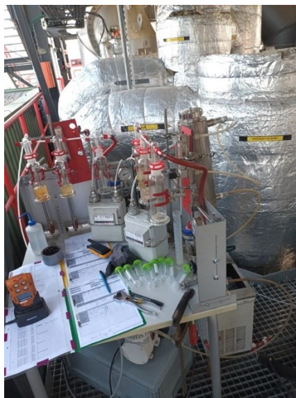
Figure 19: Setup of sampling N-compounds at the DFB gasification plant
