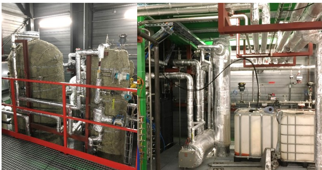
Figure 8: Fine gas cleaning (left: Fixed-bed reactors, right: Liquid based scrubber systems)
